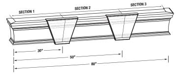
NOTE: All measurements need to be from backside.
